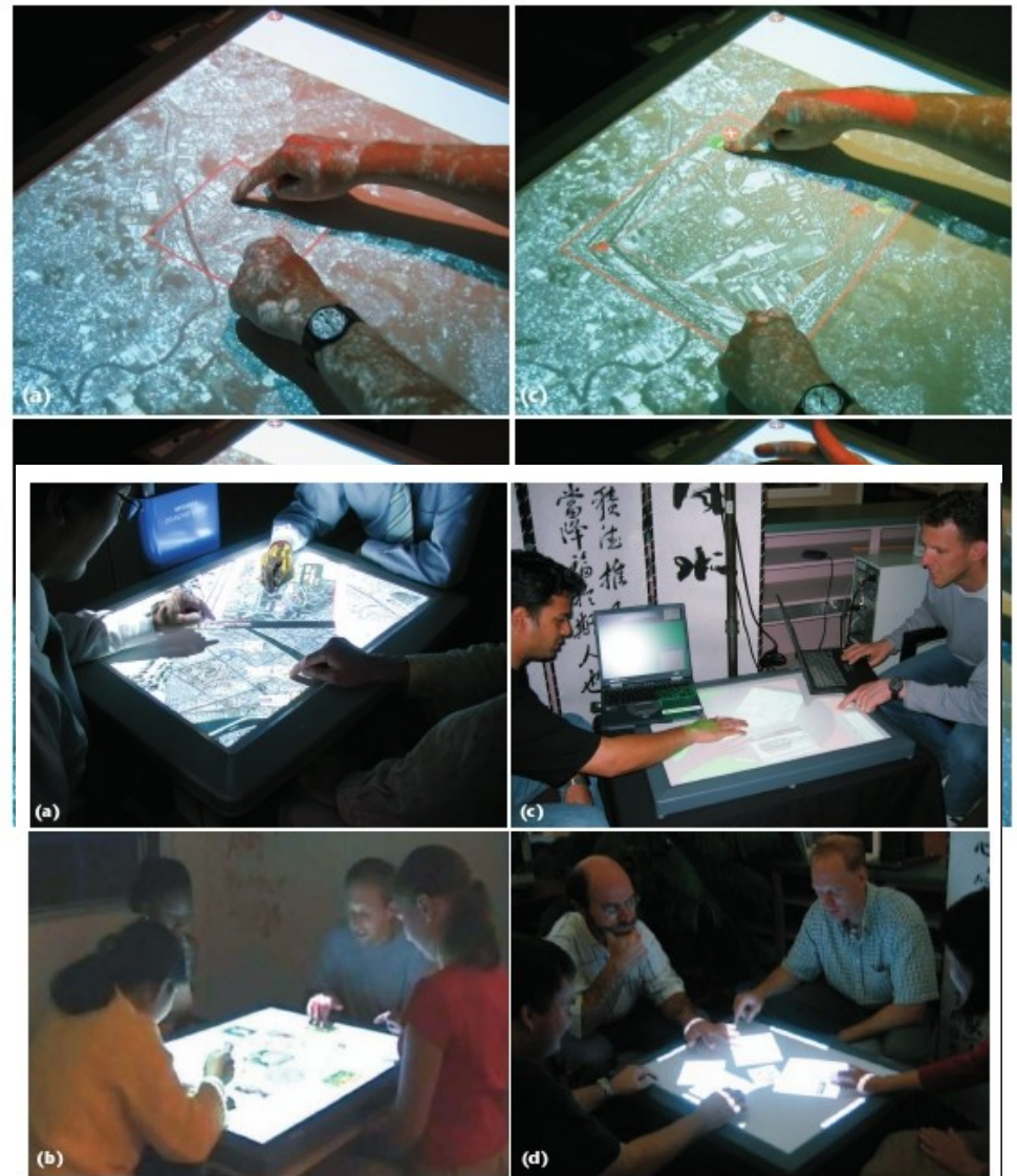
1 Tabletop iDwidgets in action: (a) DTMap, (b) TeamTag, (c) UbiTable, and (d) Table-for-N. Each application uses a MERL DiamondTouch table, which serves as an interactive tabletop.
